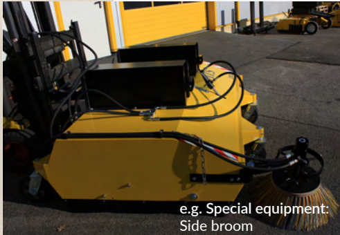
e.g. Special equipment: Side broom, water spraying device
