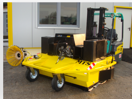
E. g. Special equipment: Reinforced vision incl. Ram protection Extra-large wheels Side broom Diesel unit Water spraying device
