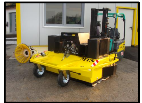
e. g. Special equipment: 2002 in reinforced vision incl. ram protection and extra-large wheels, Side broom, Diesel unit and Water spraying device
